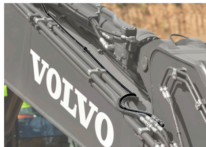
Oil drain line
