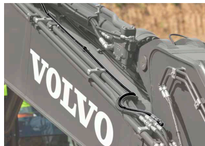
Oil drain line
